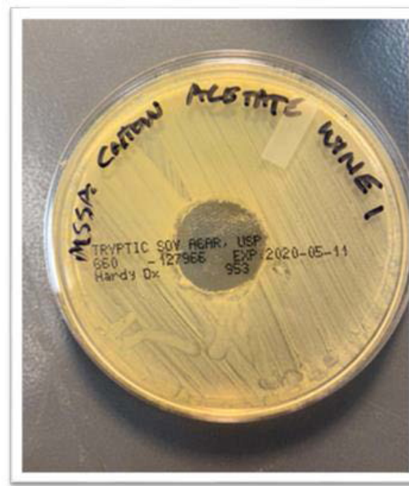
Figure 7. A nickel was the template for the samples. Then treated with S. aureus and E. coli . Zones of inhibition measured after 24 and 48 hours.
