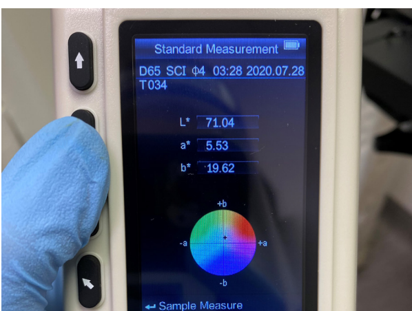
Figure 10. The colorimeter measures the sample fabric's wavelengths and intensity of light reflected off of the surface.
