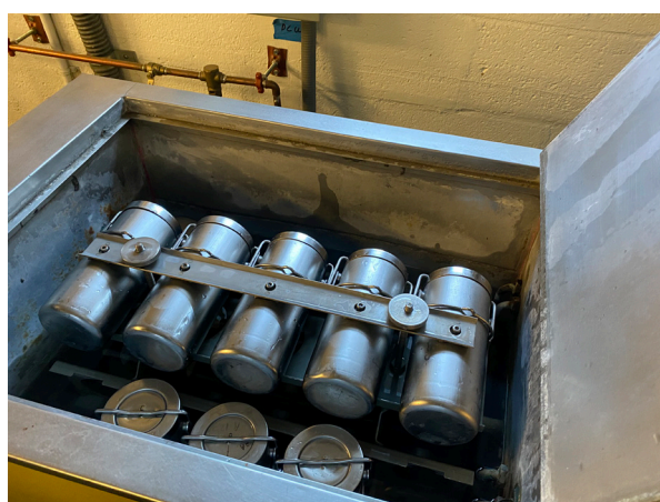
Figure 11. The lauderometer (AATCC-61) to test washing fastness of fabric samples using detergent at five cycles.
