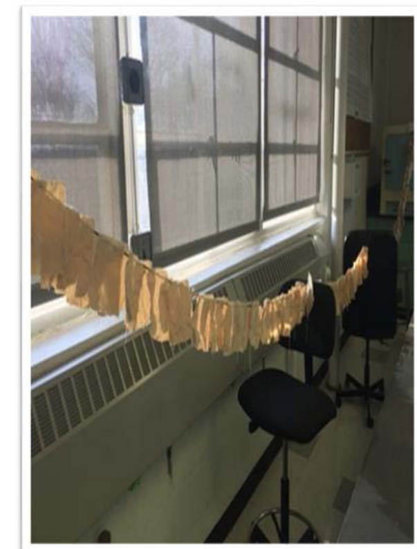
Figure 6. A 15:1 water to plant material was maintained. Cotton & wool samples were placed in a dye bath and dried for 24 hours.
