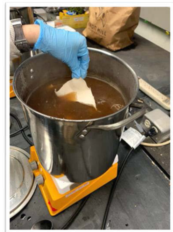
Figure 5. Cotton was mordanted with aluminum acetate, calcium carbonate, & water. Wool was mordanted with Alum, cream of tartar, & water.
