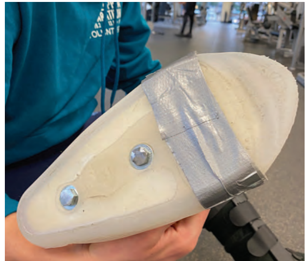
Tape to eliminate flapping that was occurring when walking
