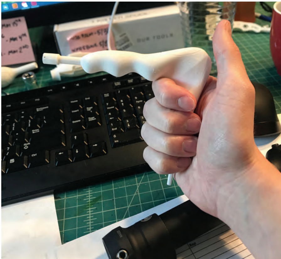
3D Print to test the ergonomics of the tool
