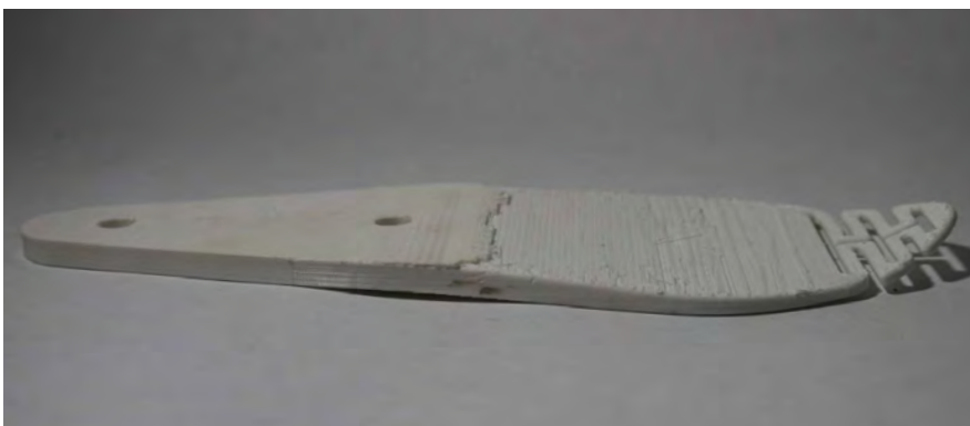
Final living hinge model, 3D print ultimately used to test stress (Permanent flex up can be seen).
