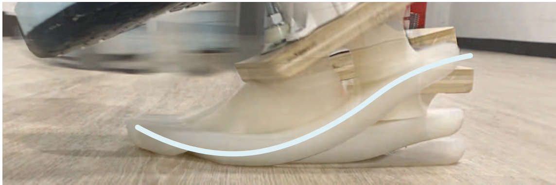
Using our empathy model to test the new cast bushings: flexing of the sole
