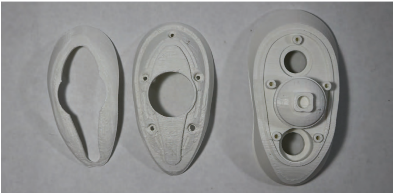
3D print, testing hole placement and split lines
