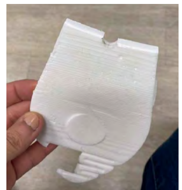
Broken toe in the cast Task 21 model
