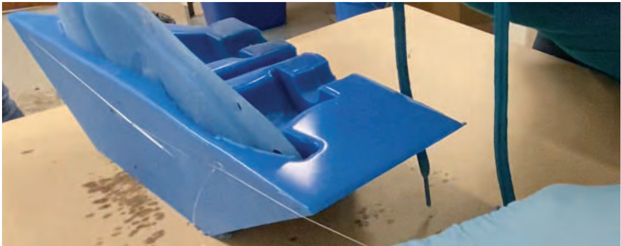
“Stitching” the threads to the mold to ensure no movement
