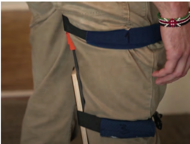
Smart Design's empathy rig, simulating the sensation of the socket around the tailbone.
