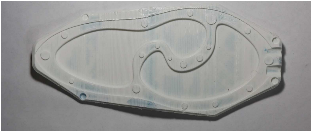
3D Printed mold for the treads
