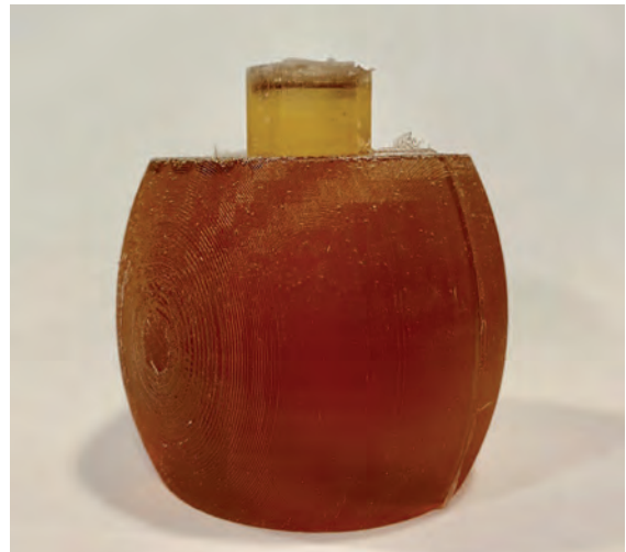
“The Bulb” cast from PMC-746
