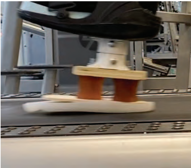
Separation occurring during walking
