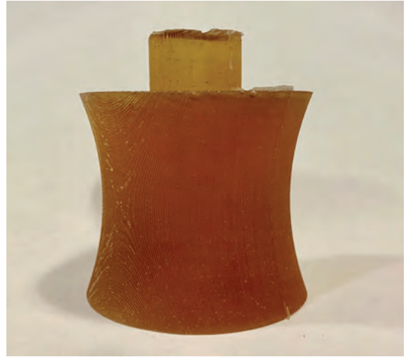
"The Hourglass" cast from PMC-746
