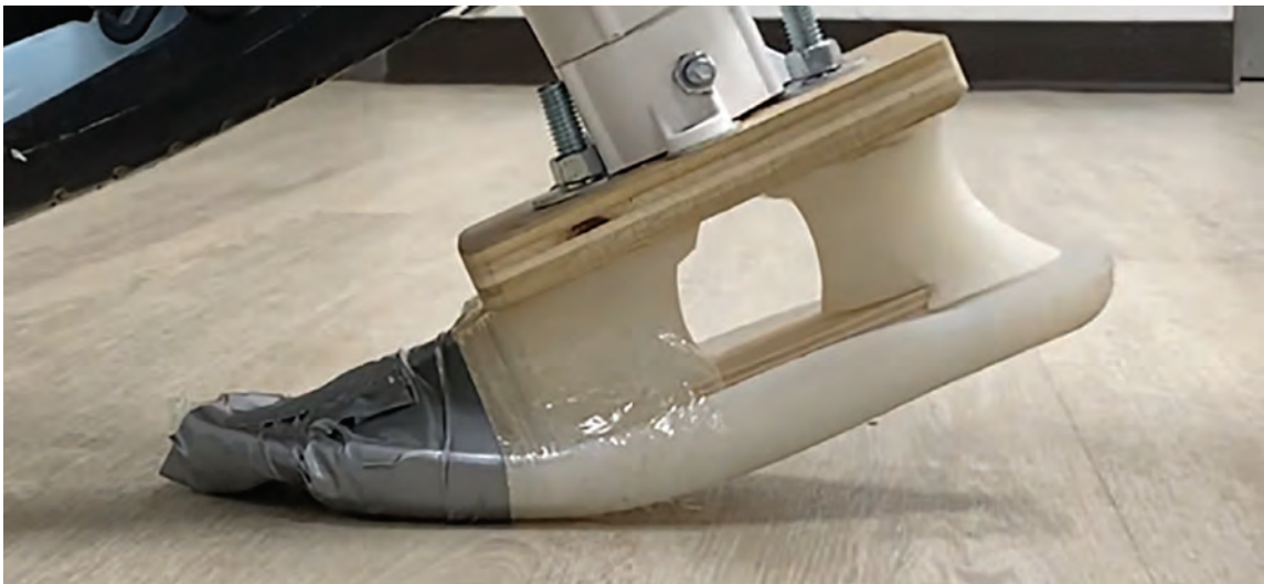
Taping the bushings to the sole created a much stronger and natural feeling when walking
