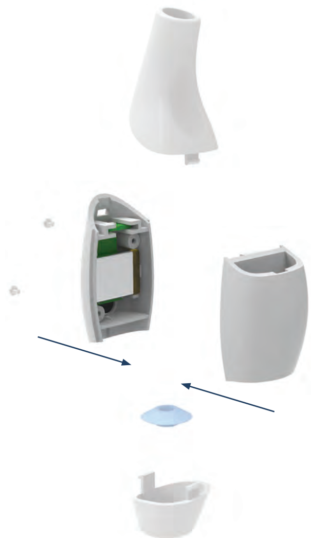
Close the front and back halves
