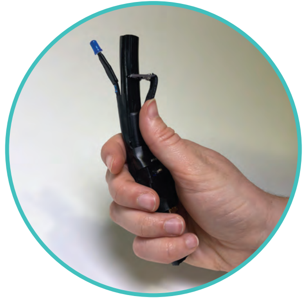
Breathing Detection Pressure Sensor
