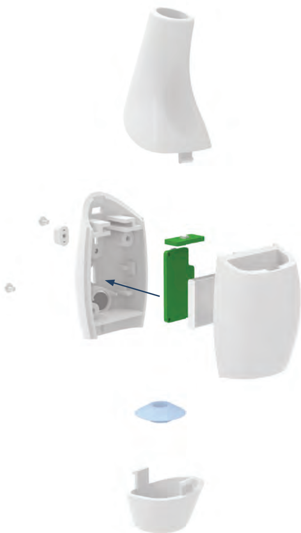
Insert the circuit board and pressure sensor
