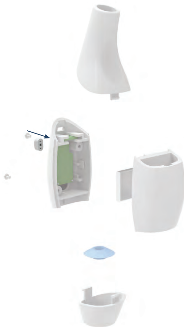
Press on the sliding switch cap
