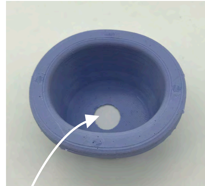
Hole to access bolt
