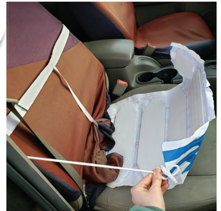
The upper strap was needed after testing, and it failed because of no support
