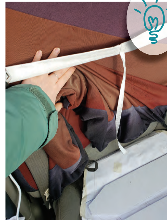
The upper strap was needed after testing, and it failed because of no support
